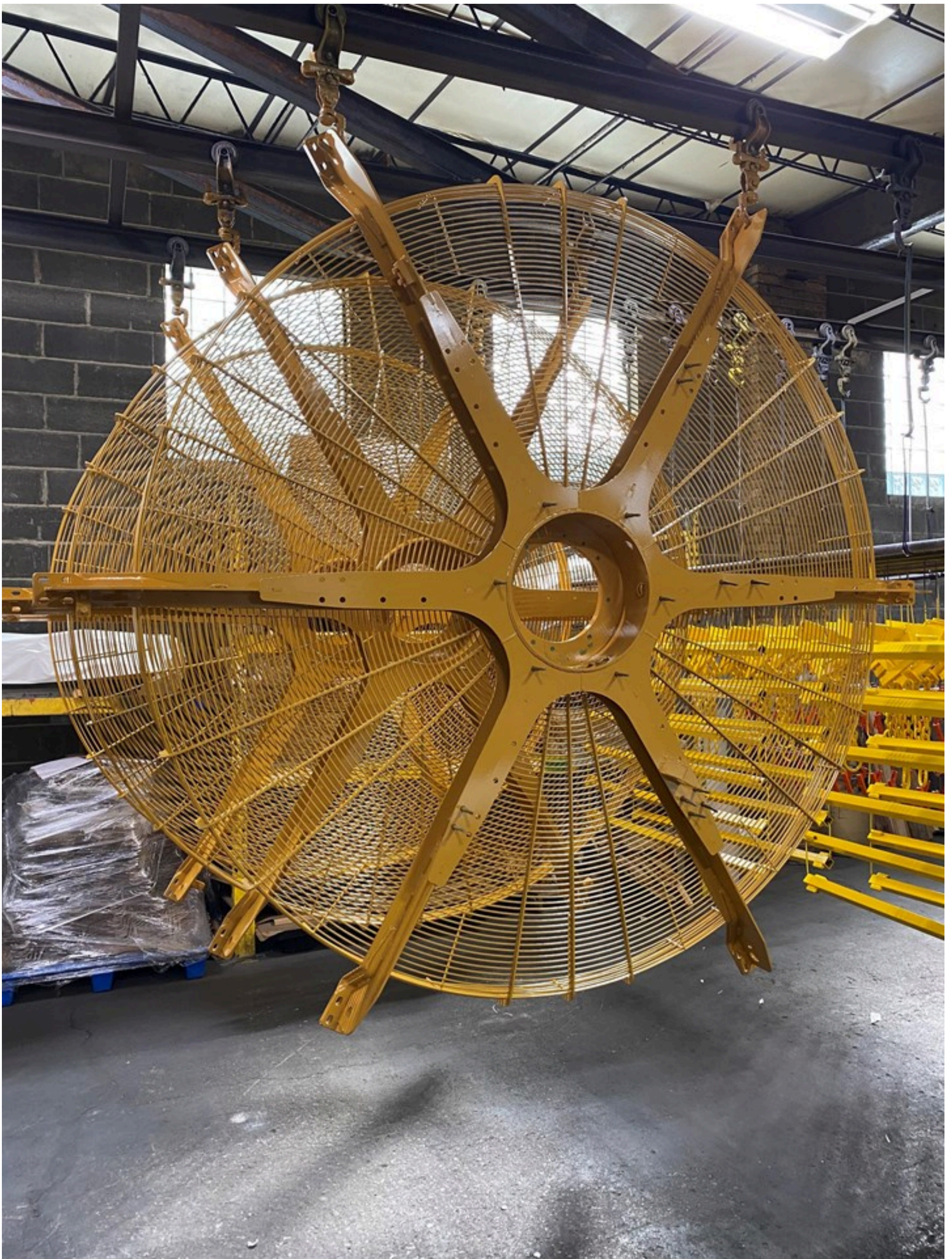
This cooling apparatus for a combine or mining equipment has been powder coated at Ace.
